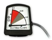
Differential pressure gauges FAD01C with potential free alarm contact allow to hook up the differential pressure control of the pre- and after-filter to the common alarm message of each dryer. In order to avoid a false error report due to start-up conditions or short-time peaks, an alarm delay can be set in the dryer control unit. The alarm message then will just be generated, if a too high differential pressure was indicated during the entire delay time interval.
